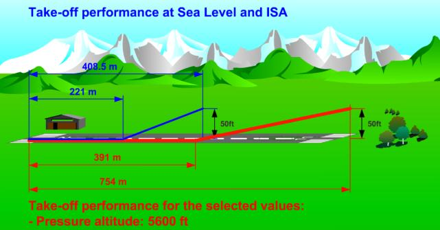
Higher density altitude means thinner air which seriously degrades aircraft performance.
