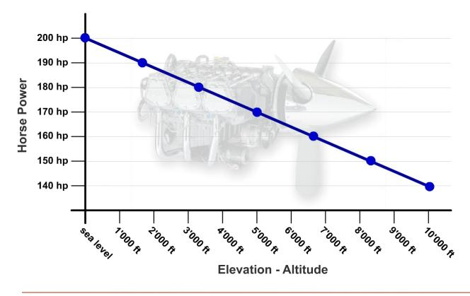
A normally aspirated engine (without a turbocharger) routinely loses about 3 % of its power for every 1000ft increase in altitude. This means that a non turbocharged Piper Arrow rated at 200 hp at sea level will generate only about 165 hp at Samedan.
