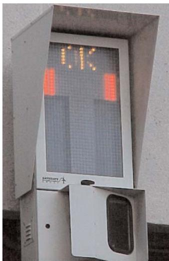
When the aircraft identification is not achieved by the system or when any obstacle is detected during the entrance into the parking position, the display will show "STOP". In this case, the ending of aircraft manoeuvre until the stop position, previous contact with TWR, will be carried out under the guidance of a FOLLOW ME vehicle.
